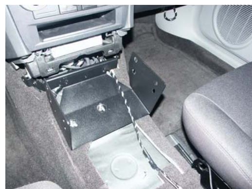
Note. To avoid crushing harness route cable over top of floor bracket
